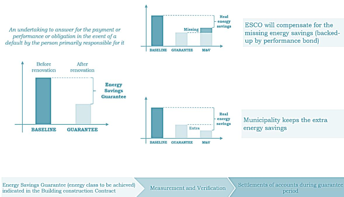
**Figure 5: Energy efficiency guarantee principle for the renovation of municipal buildings**
